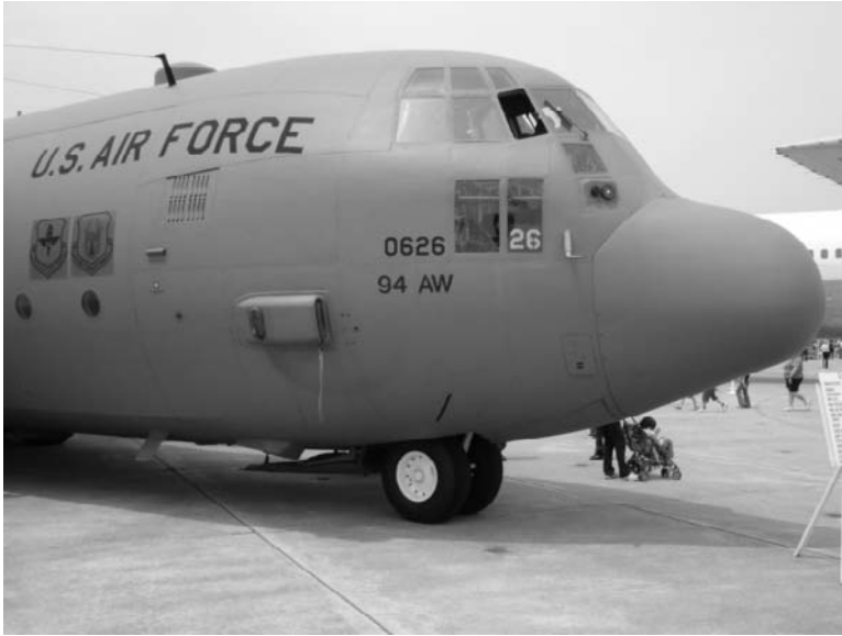
Figure 1.4 Radome-enclosed radar antenna on the nose of a modern aircraft. (Photograph courtesy of USAF National Museum.)
