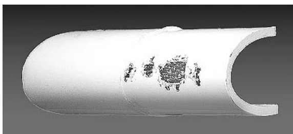
Figure 11.2 Rain erosion boot material applied to only the left half of the test article. (Photo courtesy of 3M Corporation Aerospace & Aircraft Maintenance Dept.)
