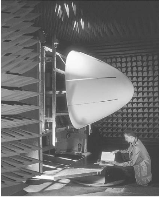
Figure 10.5 Photo of radome loss measurement in an indoor anechoic chamber. (Photo courtesy of Saint-Gobain Performance Plastics.)
