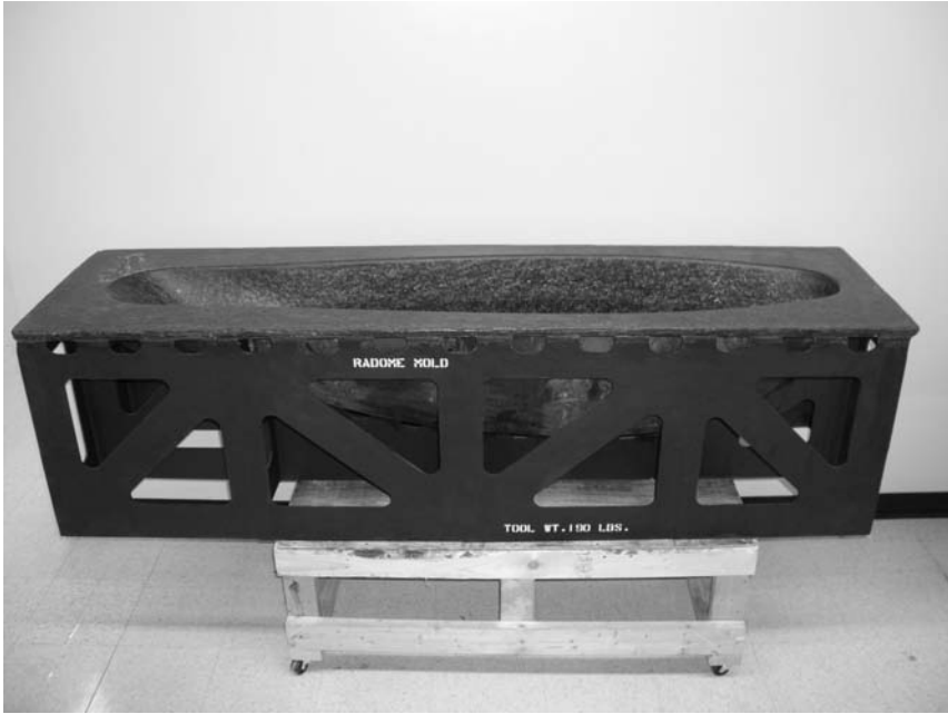
Figure 4.3 Female radome mold fixture. (Photo courtesy of Cobham Sensor Systems.)
