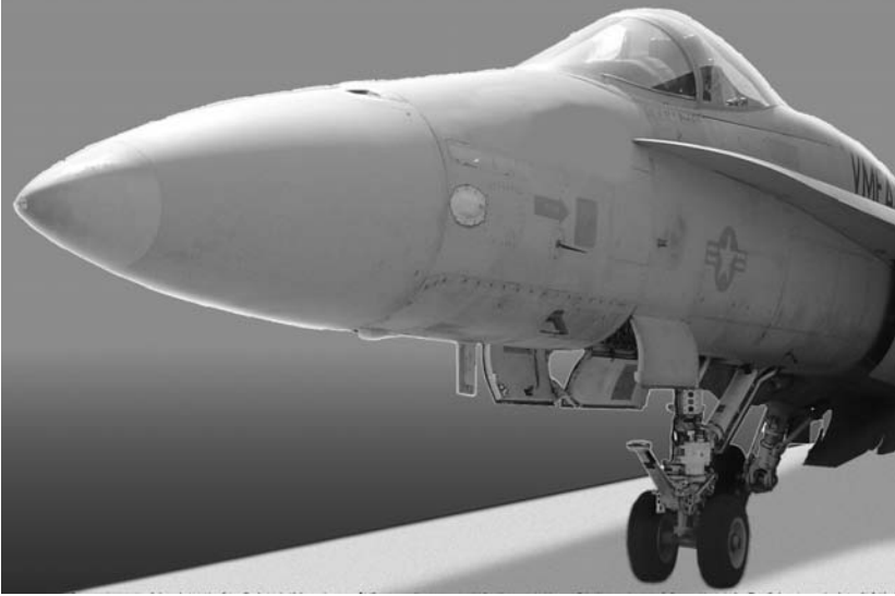
Figure 7.4 High fineness ratio tangent ogive radome used in a modern high-speed aircraft. (Photo courtesy of USDigiComm Corporation.)
