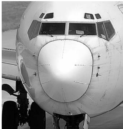
Figure 11.7 Photo of lightning diverter strips applied to an aircraft radome. (Photo courtesy of USDigiComm Corporation.)
