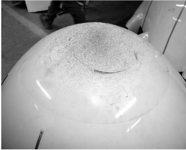
Figure 11.1 Rain erosion of a typical aircraft radome. (Photo courtesy of USDigiComm Corporation.)
