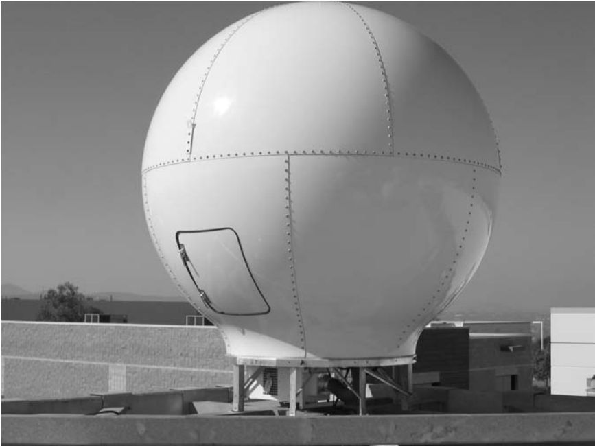
Figure 7.12 Large terrestrial radar antenna in a hemispherical radome. (Photo courtesy of MFG Galileo.)
