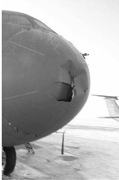
Figure 11.12 Photo of a large bird strike on aircraft radome. (Photo courtesy of Saint Gobain Performance Plastics.)
