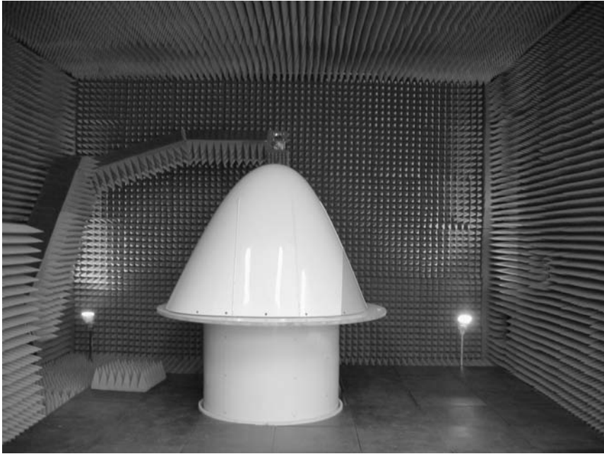
Figure 10.8 Photo of radome test in spherical near field test facility. (Photo courtesy of Orbit FR.)
