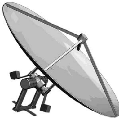
Figure 2.9 Specialized antenna gimbal that is neither AZ/EL or EL/AZ. (Photo courtesy of K. Guerin and E. Bannon of Carnegie Mellon University.)
