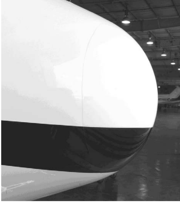
Figure 11.3 Rain erosion boot applied to an aircraft radome. (Photo courtesy of 3M Corporation Aerospace.)
