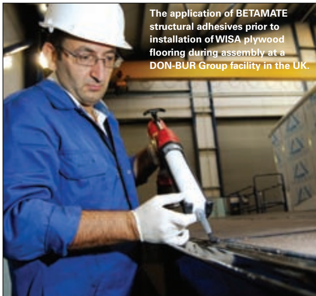
WISA plywood flooring bonded to the trailer floor using BETAMATE structural adhesives.
