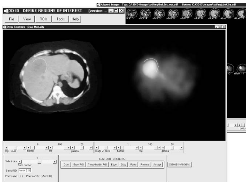
Figure 11.3. Regions of interest are defined by drawing individual contours using aligned image sets. As contours are drawn, they appear in the multi-slice, two-row, main display window (seen here behind the drawing window).
