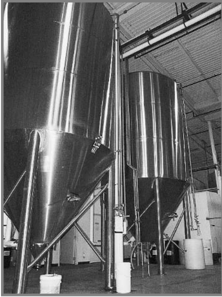
A shot of the fermentation tanks at the Milton brewery. Our original batch size was ten gallons. These tanks hold over 6,000 gallons of beer each.
