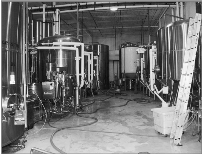
The 100-barrel tanks. The labyrinth of brewing vessels, bottling tanks, pipes and hoses that make up the fermentation hall at the Milton brewery.
