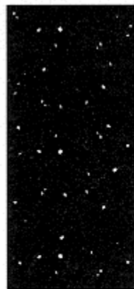
Fig. 3 Details of a double-split experiment performed with electrons. Interference patterns were once thought of as evidence for wave motion. However, close observation of detail shows that the electrons arrive in individual lumps. In the left illustration so few electrons have arrived that we see an almost random pattern of bits. The illustrations to the right show what happens as the exposure becomes longer: more and more electrons arrive until eventually the familiar interference pattern becomes visible.
