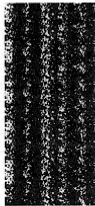
Fig. 3 Details of a double-split experiment performed with electrons. Interference patterns were once thought of as evidence for wave motion. However, close observation of detail shows that the electrons arrive in individual lumps. In the left illustration so few electrons have arrived that we see an almost random pattern of bits. The illustrations to the right show what happens as the exposure becomes longer: more and more electrons arrive until eventually the familiar interference pattern becomes visible.
