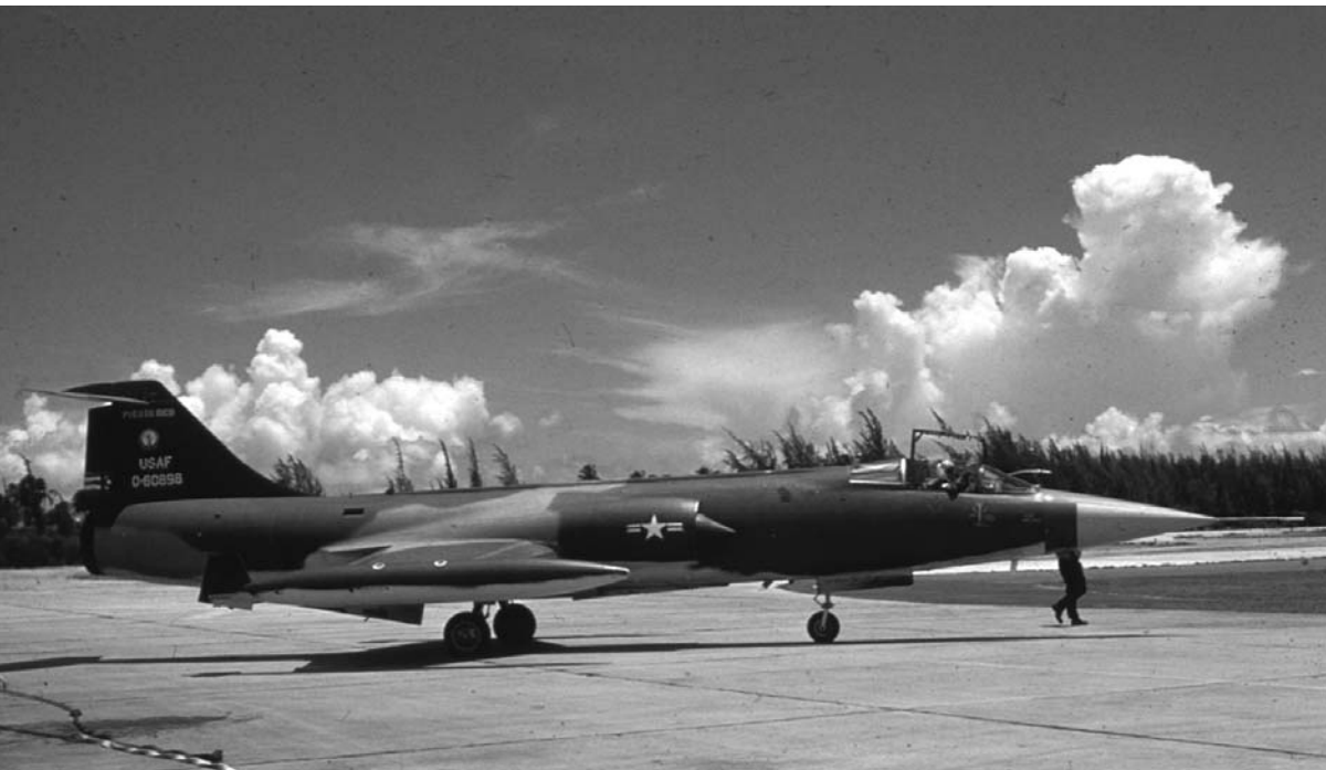
Lockheed’s “missile with a man in it” shown in Vietnam-era camouflage and flown by the Puerto Rican Air National Guard. The F-104 Starfighter was an ideal interceptor, but saw only limited duty in Southeast Asia. Notice the extremely short, stubby wings. Courtesy Candid-Aero Files.
