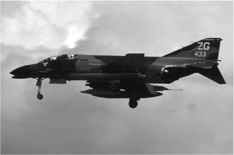
An F-4C Phantom II with an SUU-16 gun pod suspended from the centerline hard point. The SUU-16 is a 20-mm Gatling gun capable of firing up to six thousand rounds of ammunition a minute. Courtesy JEM Aviation Slides.
