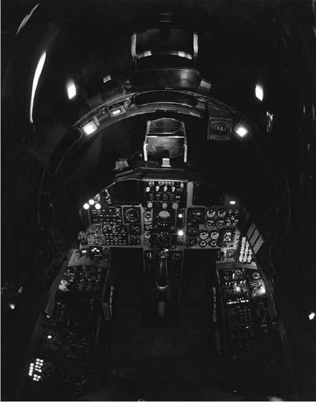
Cockpit of the F-15A Eagle. Notice the head-up display, rearview mirrors, well laid-out instrument panel, and excellent visibility. Courtesy The Boeing Company.
