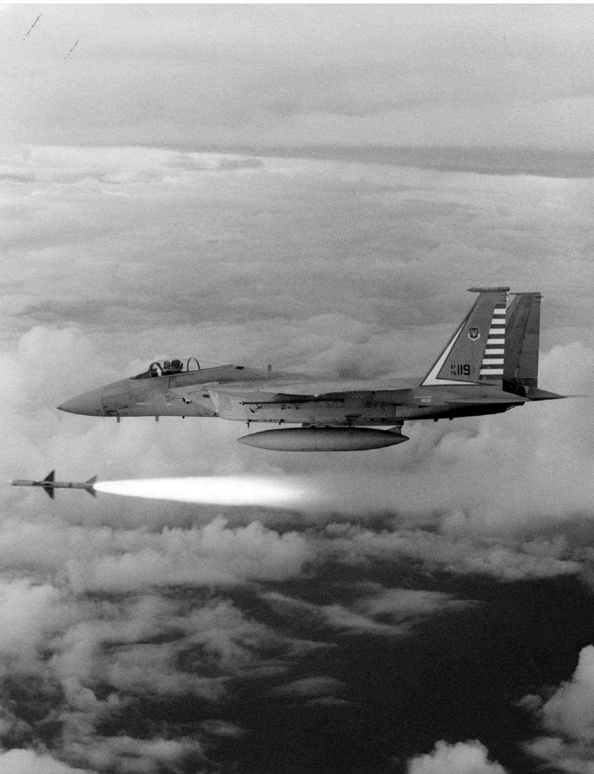
An F-15A launches an improved AIM-7F Sparrow missile. The Sparrow is a radar-guided missile. Courtesy The Boeing Company.
