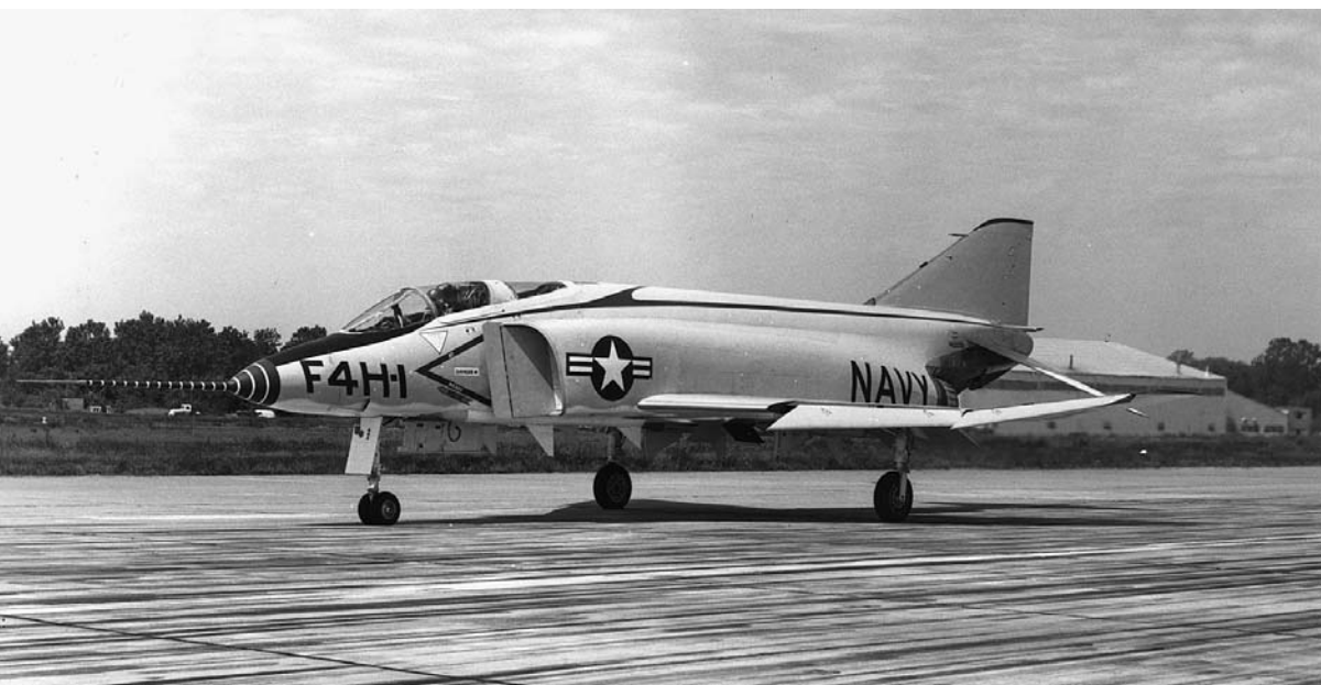
The first of more than five thousand. McDonnell's first production F-4 Phantom II undergoing taxi tests. Note that the main landing gear doors have been removed. Courtesy The Boeing Company.
