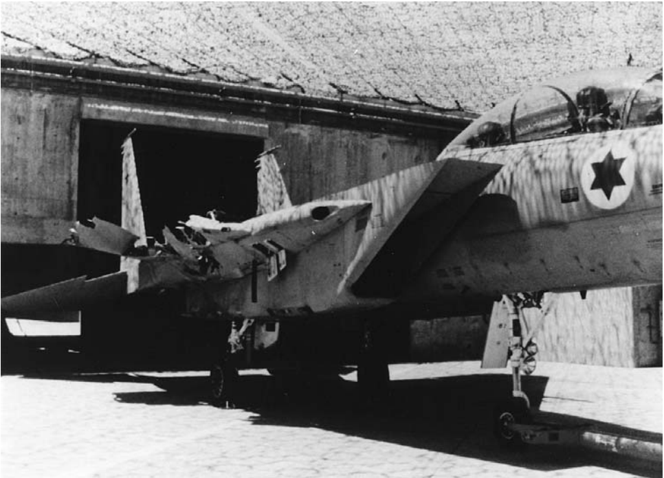
Perhaps the greatest benefit of a “fly-by-wire” control system is survivability. This Israeli F-15 Eagle suffered a midair collision that sheared the entire right wing from the airplane outboard of the wing root. The pilot flew back to his base on one wing and made a safe landing. The airplane only needed new tires, brakes—and a right wing before returning to duty. Courtesy The Boeing Company.
