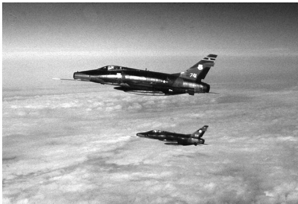
Two Air National Guard F-100D Super Sabres in formation above the clouds. The “Hun” was the world’s first production aircraft to achieve sustained supersonic flight, but it was not nearly as maneuverable as its predecessor, the F-86 Sabre. The D-model aircraft, as shown here, was developed for the ground-attack mission only. In the Vietnam War, F-100Ds flew 344,619 combat and combat-support sorties, mostly in South Vietnam. Courtesy JEM Aviation Slides.
