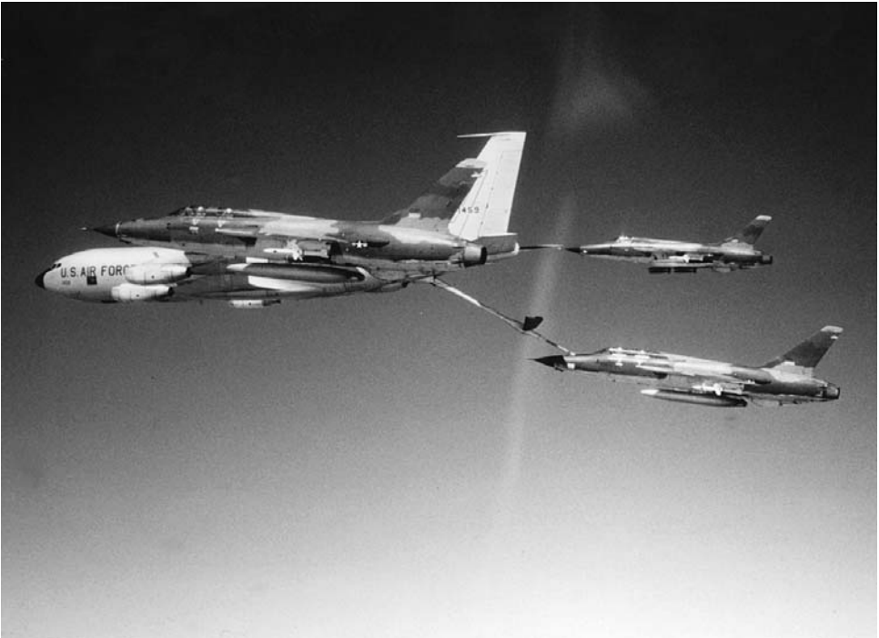
An Iron Hand strike force refuels before entering North Vietnam. The two F-105Fs in the foreground carry AGM-45 Shrike missiles that seek enemy radar frequencies and then follow the signal to its source. The F-105D in the background carries a load of conventional bombs to finish destroying the SA-2 site. These hunter-killer teams were quite effective in protecting the main strike force from the SAMs. Courtesy Alton Meyer, via Jim Ray.
