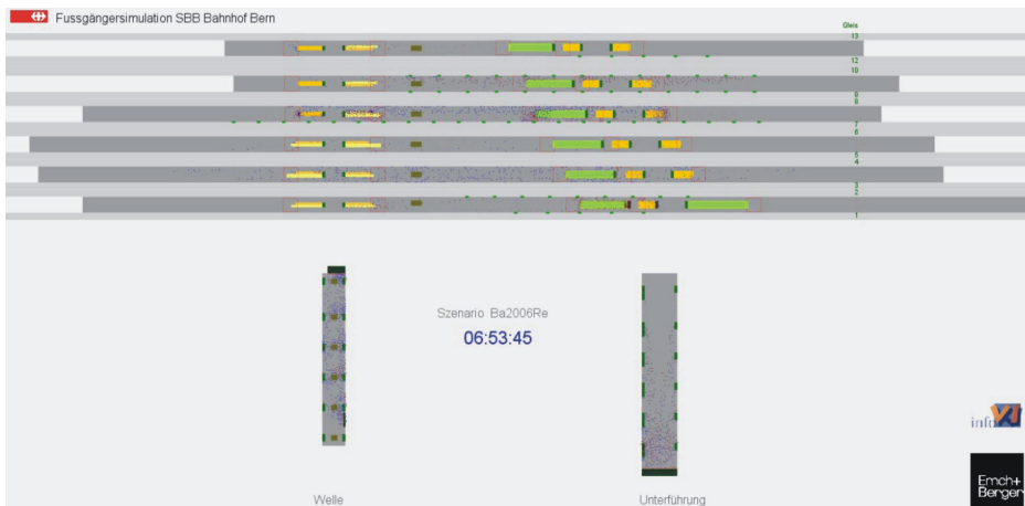
Fig. 1. Scenario 2006Re : Layout of 2006, without renovated overpass. Larger dark areas represent the entries/exits of the railway station, smaller dark areas are the transfer areas connecting areas that should be on the same level. Tracks are light gray; platforms are framed by thin black lines.
