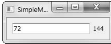
Figure 3.5 A custom class multiplies the input received through a custom slot by 2 and emits the result through a signal.
