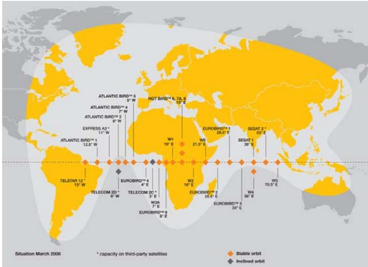
Fig. 1. The Eutelsat satellites on the geostationary arc
