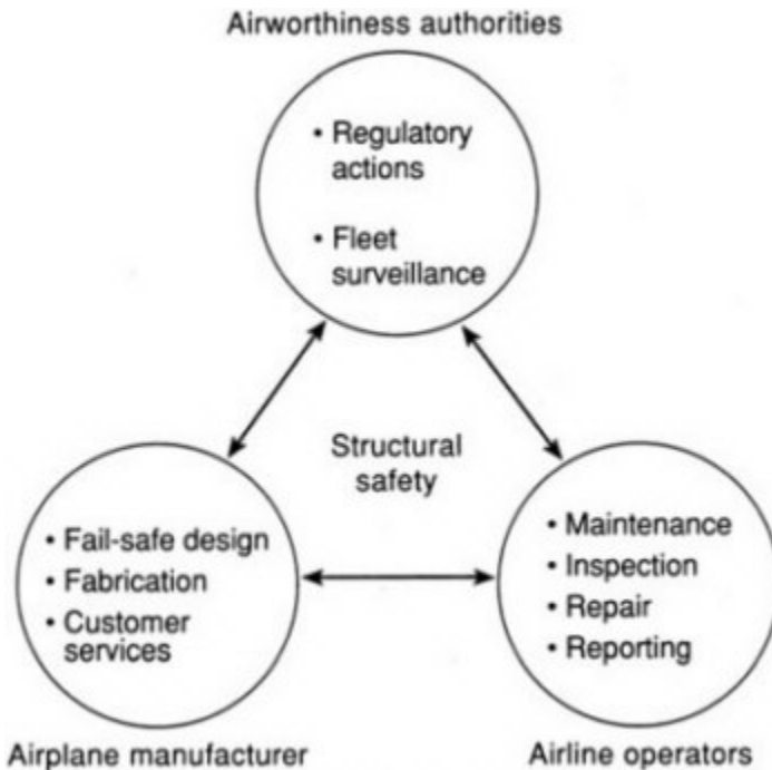
FIGURE 2 Airplane transportation system. SOURCE: The Boeing Company.
