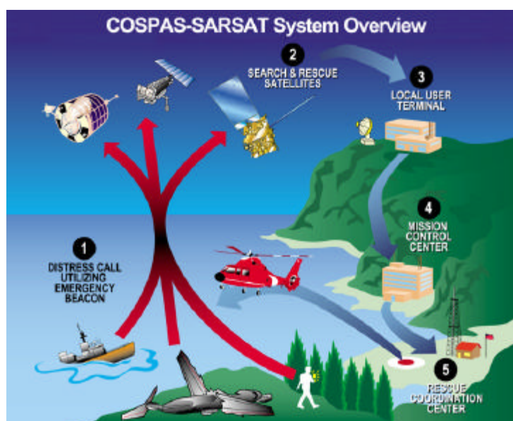
Figure 2 The Search and Rescue Satellite Aided Tracking (SARSAT) system uses NOAA satellites in low-earth and geostationary orbits to detect and locate aviators, mariners, and land-based users in distress. SOURCE: NOAA National Environmental Satellite, Data, and Information Service. http://www.sarsat.noaa.gov/
