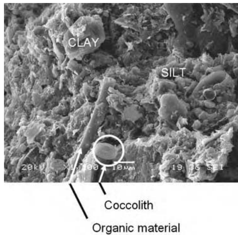
Figure 6.5. Scanning electron microscopy analysis of natural dredged material
