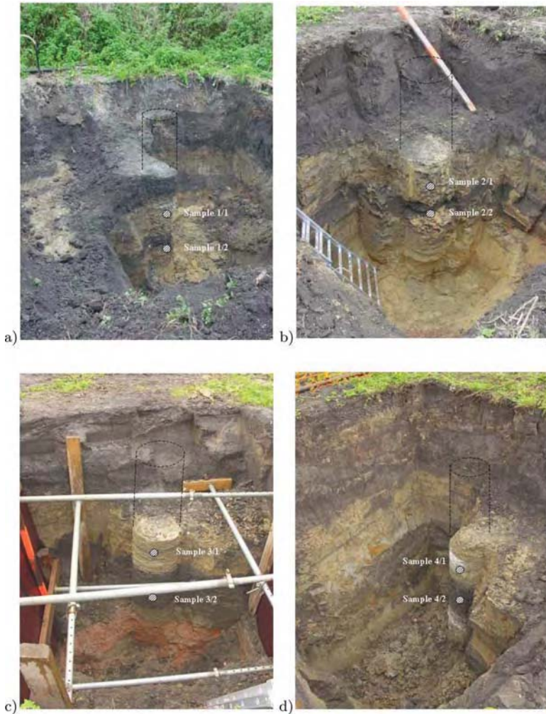
Figure 8.14. Partial excavation of trial columns (a) No. 1 mixed with 85 \text{ kg/m}^3 of L/C-100/0 (b) No. 2 mixed with 130 \text{ kg/m}^3 of L/C-0/100 (c) No. 3 mixed with 130 \text{ kg/m}^3 of L/C-50/50 and (d) No. 4 mixed with 170 \text{ kg/m}^3 of L/C-100/0; all implementing CEM II/B-M 32.5
