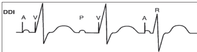
Fig. 4.16. DDI mode will pace and sense both atrium and ventricle. This eliminates the competition with intrinsic atrial beats as seen with the second P-wave. The P-wave is sensed and inhibits the atrial output, but does not start an AVI as would happen in a DDD system. The ventricular output will occur at the proper time to maintain the programmed pacing rate.
