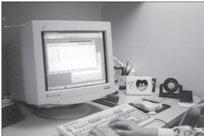
Fig. 9.2. Typical transtelephonic receiving center. This Paceart™ system is computer based and runs on a standard “PC”. Analysis, reporting and storage of the transmitted rhythm strip is performed efficiently as opposed to the “cut and paste” method of the older style heated pen strip recorders.
