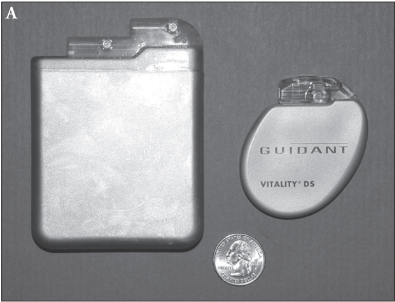
Fig. 13.1. Picture of old and new ICDs front (a, above) and profile (b, below). Note the marked decrease in size that has occurred over the past 10 years.
