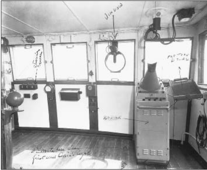
The Stockholm 's wheelhouse, which had been overseen by the third mate, Johan-Ernst Bogislaus August Carstens-Johannsen, in the hours before the collision. The radar set, toward right, is next to a board used to plot an oncoming ship's changing position. (Archives of Haight, Gardner, Holland & Knight)
