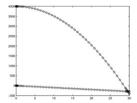
The bottom line shows velocity starting at zero and dropping linearly. The top line shows position starting at 4000 m and dropping parabolically (but remember that this parabola is a function of time, not a ballistic trajectory).
