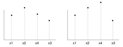
If  $f(x_4)$  is less than than  $f(x_2)$  (shown on the left), then the new triple  $(x_1, x_2, x_4)$  brackets the maximum. If  $f(x_4)$  is greater than  $f(x_2)$  (shown on the right), then  $(x_2, x_4, x_3)$  brackets the maximum. Either way the range gets smaller and our estimate of the optimal value of x gets better.
