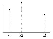
This diagram show that we have evaluated f in three places,  $x_1$ ,  $x_2$  and  $x_3$ , and found that  $x_2$  yields the highest value. If f is continuous, then there has to be at least one local maximum between  $x_1$  and  $x_3$ , so we would say that the triple  $(x_1, x_2, x_3)$  brackets a maximum.
