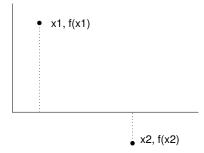
We are given a function, f, that we can evaluate, and we want to find a root of f; that is, a value of x that makes f(x) = 0. If we can find a value,  $x_1$ , that makes  $f(x_1)$  positive and another value,  $x_2$ , that makes  $f(x_2)$  negative, then there has to be a root in between (as long as f is continuous). In this case we say that  $x_1$  and  $x_2$  "bracket" the root.
