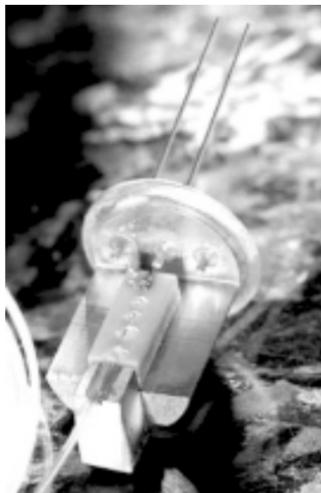
**Figure 5.21.** Fiber pigtailed module using precision-machined substrate for laser-to-fiber passive alignment.<sup>[52]</sup>
