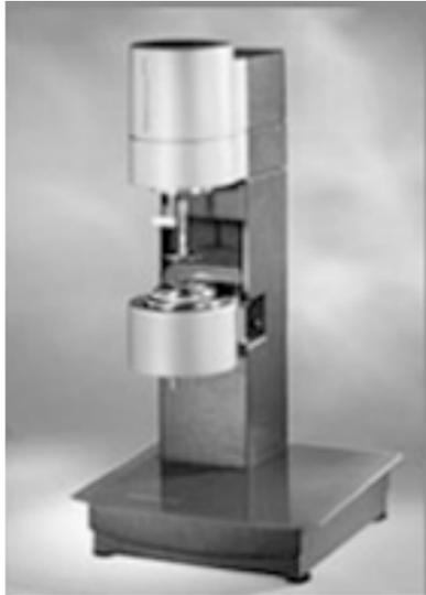
**Figure 7.2.** Haake viscometer.
