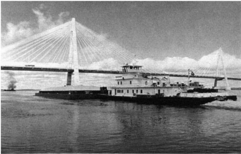
Plate 2.3 On the Parana river in Paraguay, a low-draught, high capacity push-tug and barges was introduced in 1995 by the international Cargill company to move grain for export (Photo: Cargill plc).
