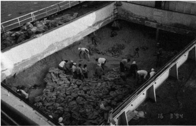
Plate 7.2 Cuban bulk sugar, hand bagged for unloading at Alexandria—a labour intensive, slow method of cargo handling which characterises many Third World ports (Photo: Cargill plc).
