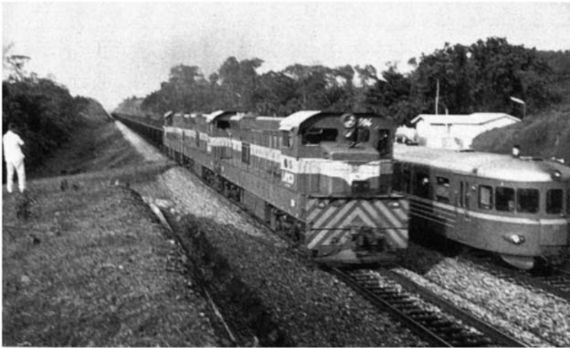
Plate 3.1 In Liberia, the LAMCO railway is of high design standards, allows 9,000-tonnes ore trains and provides passenger and general freight transport.
