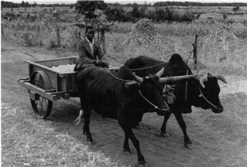
Plate 5.4 The Intermediate Technology Development Group has designed a variety of vehicles, such as this ox-cart in Kenya, which can be easily produced locally with available materials but greatly increase transport efficiency (Photo: Intermediate Technology/Jeremy Hartley).
