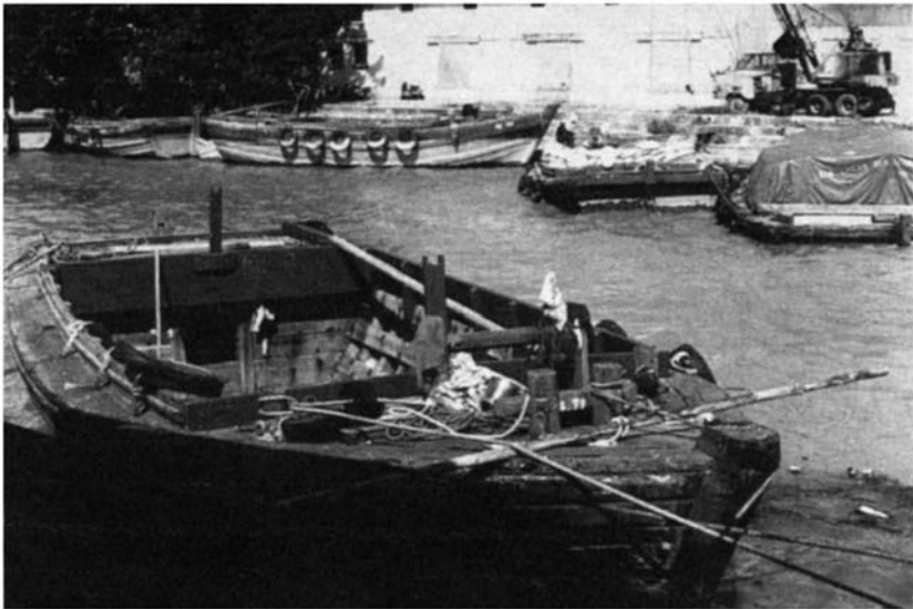
Plate 7.1 The use of lighters in roadstead ports such as Malacca, Malaysia, involves double handling and restricts the volume and type of cargo that can be dealt with.
