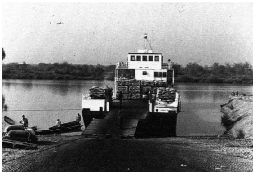
Plate 2.4 A simple ramp allows ease of loading palletised rice by fork-lift truck at Ghana's Volta Lake port at Yapei, but on waterways of variable depth more sophisticated solutions may be necessary.
