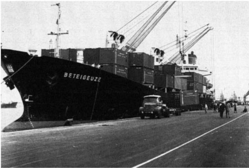
Plate 7.3 The use of 'self-sustaining' container ships makes costly port container cranes unnecessary but is only suitable when the number of containers is small.
