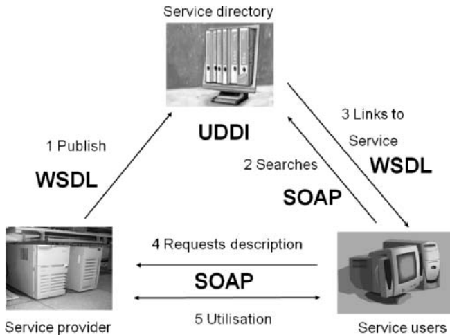
Figure 2: Web Service based SOA, excerpt from: Dostal et al. (2005), p. 28.
