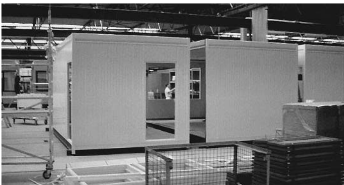
Plate 3 Prefabricated modular units at the De Meeuw factory
