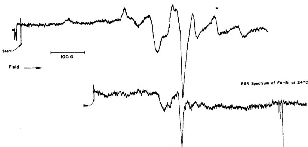
Figure 7 Solid state ESR spectra of hydrophilic fraction A-1 and hydrophobic fraction B-1 at 24 \pm 1^\circ\text{C} .
