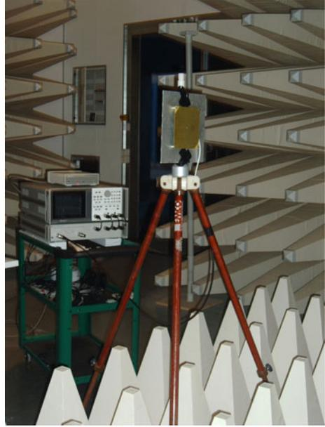
**Fig. 6.4** Antenna measurements performed in anechoic chamber [5]
