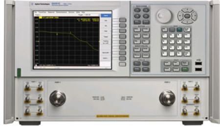
The FDR approach is often used for the dielectric spectroscopy of materials and for impedance characterization of electronic devices and components. In particular, a VNA used in conjunction with a dielectric probe kit can be employed to characterize the dielectric behavior of materials. However, it is important to point out that, although these are well-established experimental setups, their application is far from being universal, and often specific solutions must be designed.
