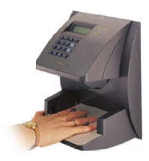
Figure 7-4 Verifying identity through hand geometry. Courtesy: HID Corporation.
