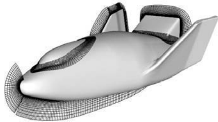
Fig. 3. X38 Crew Return Vehicle with several of its computational body grids
