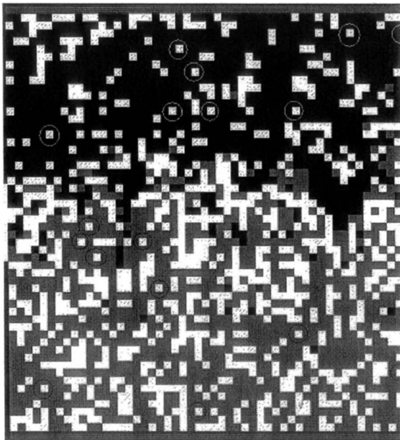
Figure 5.3. A cellular automata model of the interface between two immiscible liquids, after the demixing process has reached an equilibrium. A solute (encircled cells) has partitioned into the two phases according to its partition coefficient
