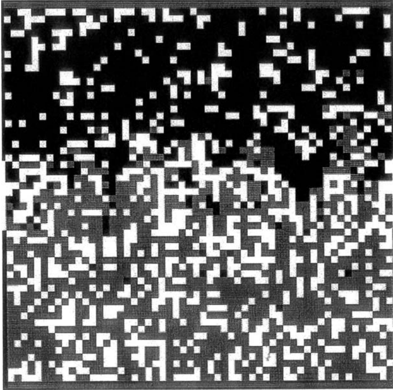
Figure 5.2. A cellular automata model of the interface between two immiscible liquids, after the demixing process has reached an equilibrium
