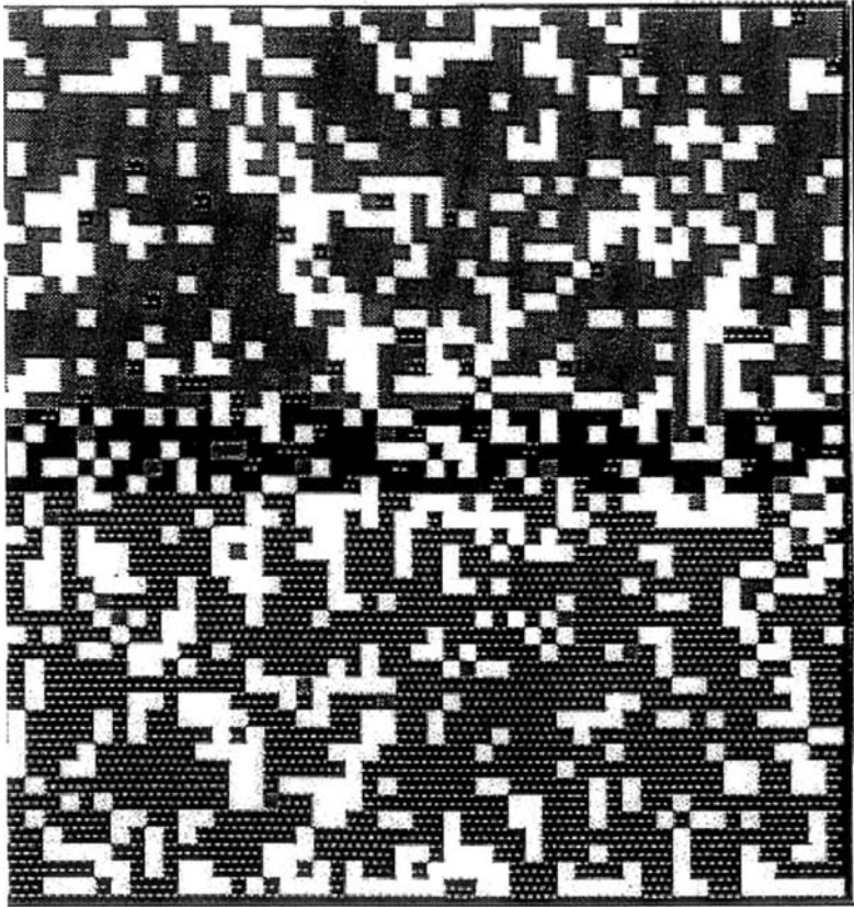
Figure 6.4. Model of a membrane (center horizontal layer of cells) separating two regions of the grid, both being water
