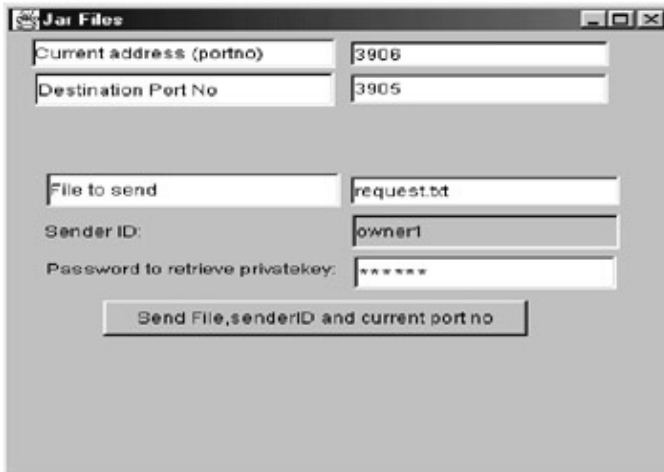
Figure 5: Sending an authentication request to the host When the sending party receives the signature and request.txt, these will be automatically authenticated (Figure 6). In this way, the sending party can be sure whether the destination host is a genuine or a bogus one.
