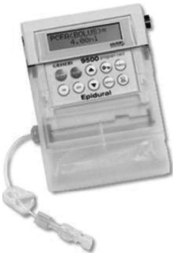
Figure 3.4 Apparatus for patient-controlled epidural analgesia (PCEA)
