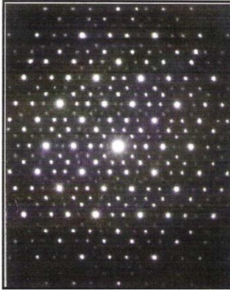
**Fig. 10.5.** The Diffraction pattern of an icosahedra quasi crystal
