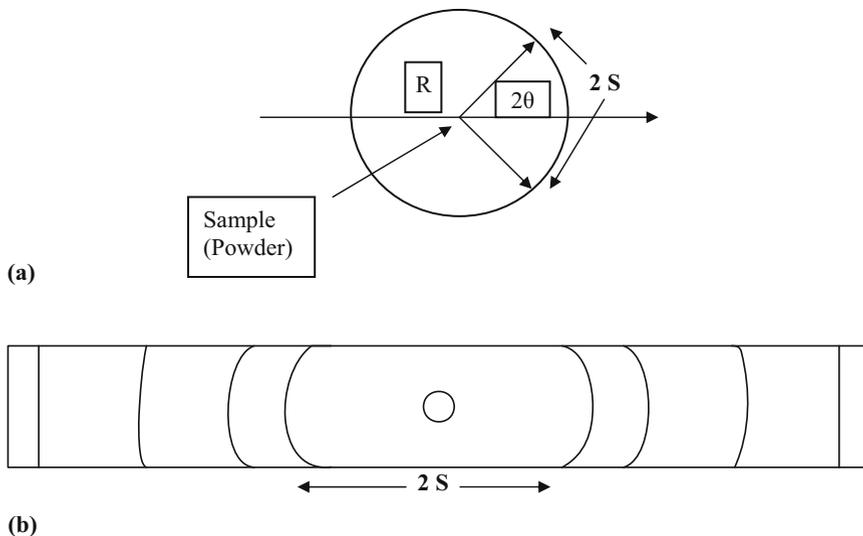
**Fig. 7.16.** (a) The Debye–Scherrer cylindrical camera and incident monochromatic  $K_{\alpha}$  radiation. (b) The cylindrical film and Debye arcs from various planes
