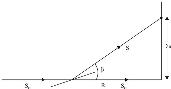
Fig. 7.6. Diffraction of X-ray in rotation/oscillation camera
