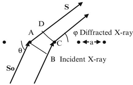
Fig. 6.5. X-ray diffraction from the rows of atoms/molecules
