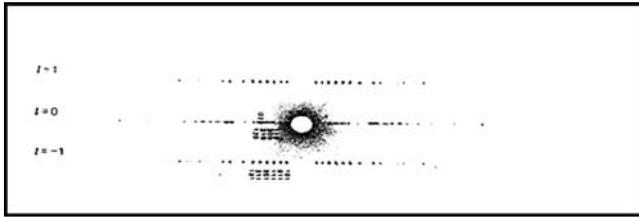
**Fig. 7.5.** The oscillation photograph of a single crystal mounted along its  $c$ -axis (By courtesy of L.S. Dent Glasser)
