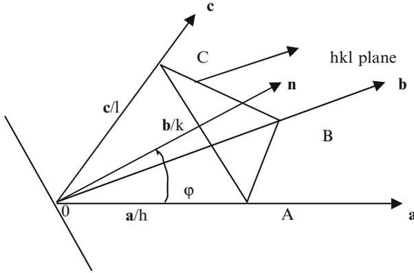
**Fig. 6.8.**  $OA$ ,  $OB$ , and  $OC$  are the intercepts on the  $\mathbf{a}$ ,  $\mathbf{b}$ , and  $\mathbf{c}$  axes of the plane  $hkl$ ,  $\mathbf{n}$  is the unit vector normal to the plane  $hkl$  and  $\varphi$  is the angle that this unit vector makes with the  $\mathbf{a}$ -axis
