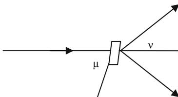
Then, the distance through which the film is to be moved back and the formulae relating to the recording of upper layer are given as: For zero layer arrangement  $\mu = \nu = 45^\circ$ , layer screen subtends  $90^\circ$  cone at the crystal, and this is to be kept constant. The upper layer is to be recorded by changing  $\mu$ . Now for  $n$ th layer,
