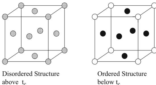
**Fig. 10.3.** Atomic sites having random occupancy by either Au or Cu atoms in disordered structures. *Filled circle*, atomic sites occupied by Cu atoms; *open circle*, atomic sites occupied by Au atoms
