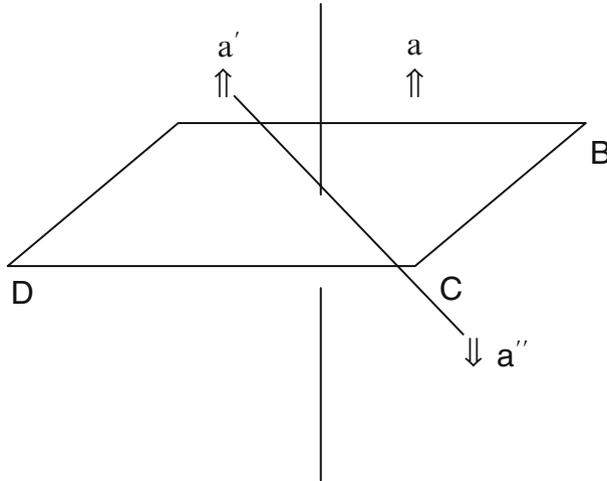
**Fig. 3.8.** Equivalence of  $\bar{2}$  and  $m$  a to  $a'$  by a twofold rotation and then inversion to  $a''$ . These entire operations are equivalent to a simple mirror reflection over the plane ABCD (a changes directly to  $a''$ )
