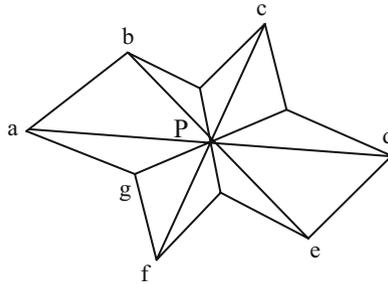
**Fig. 3.6.** An irregular polygon has a centre of symmetry at the point P. Each point is equidistant from P, from the corresponding point on the opposite side of centre point P. If every point within a body can be inverted through a centre then the body is transformed to self coincidence by the inversion
