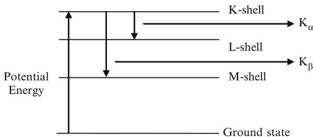
**Fig. 6.1.** Emission of  $K_{\alpha}$  and  $K_{\beta}$
