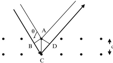
Fig. 6.6. Bragg's reflection from a set of  $hkl$  planes having interplanar distance  $d$
