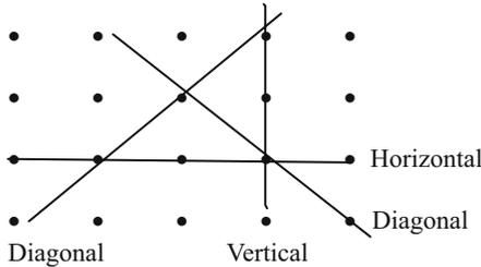
**Fig. 3.4.** Four mirror planes in a plane lattice
