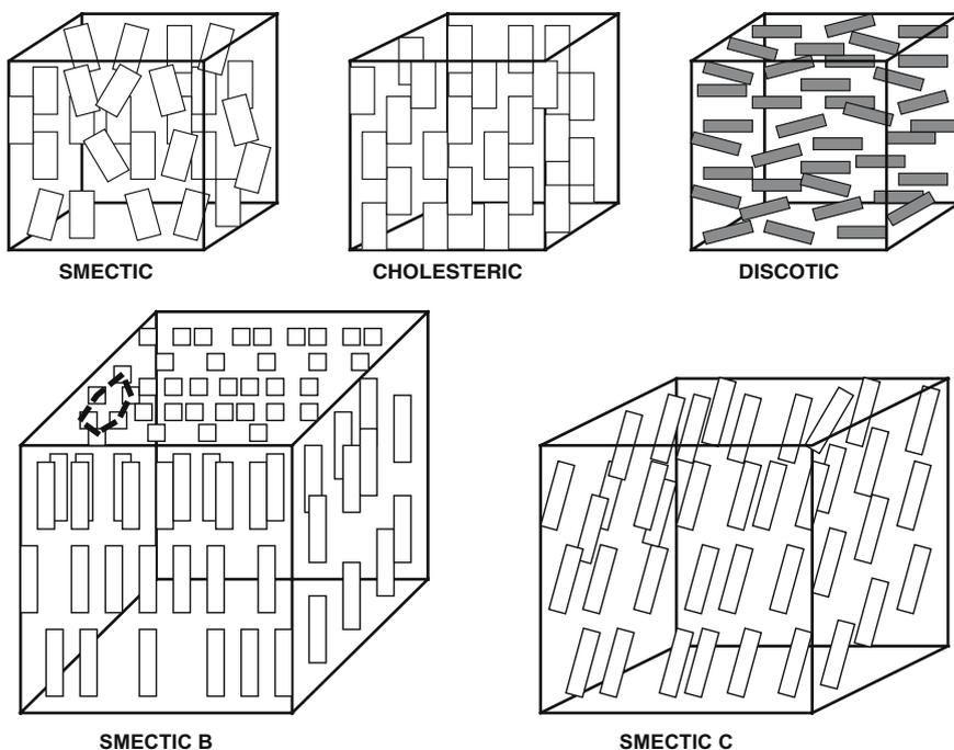
**Fig. 10.10.** Smectic B and smectic C liquid crystals
