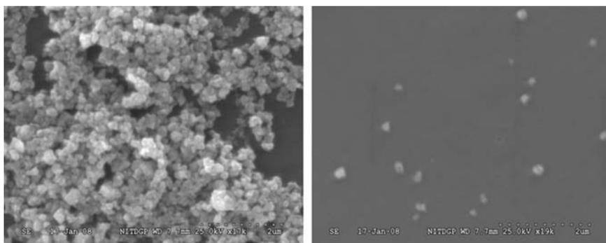
**Fig. 10.19.** Scanning electron micrograph of nanocrystalline Nickel ferrite sample prepared by chemical route with ball – milling time of 1 h. The picture indicates that the grains are well resolved and have almost spherical in shape. The particle sizes are varying between 20 and 50 nm. Figure on the left indicates that the small particles are getting agglomerated and the figure on the right indicates the single particle picture. By courtesy of S. Ghatak and A.K. Meikap (unpublished work)
