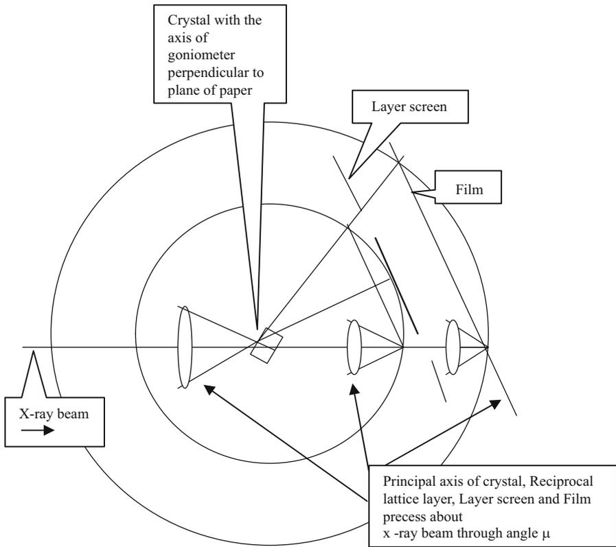
**Fig. 7.14.** Zero layer setup for Buerger precession camera
