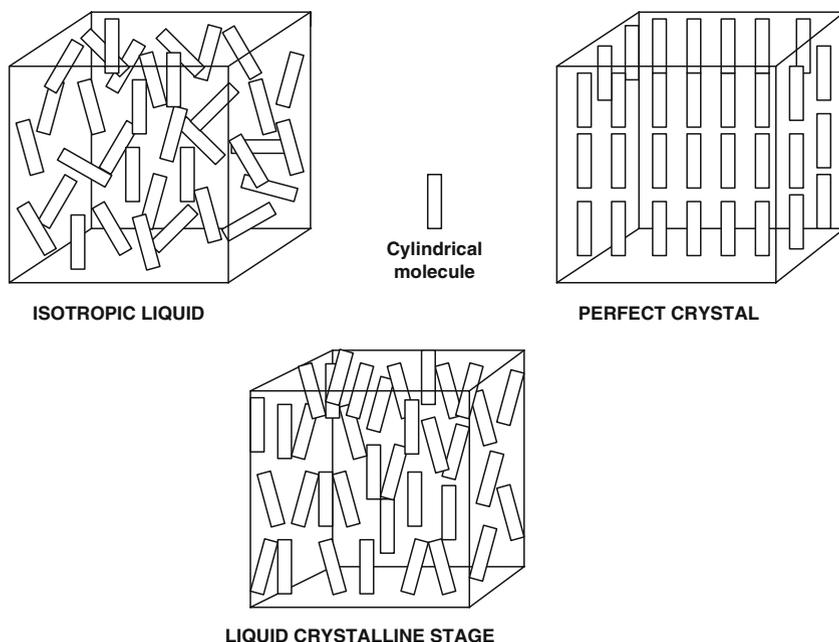
**Fig. 10.9.** The states of isotropic liquids having random arrangement of cylindrical molecules in space, the ordered arrangement (positional and rotational) of the molecules in perfect crystalline stage, and an intermediate stage, that is, liquid crystalline stage
