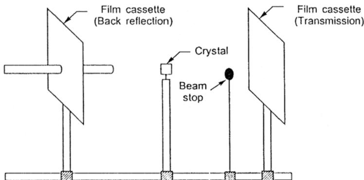
**Fig. 7.1.** Laue pin-hole camera. Single crystal is stationary and two flat fixed films for recording transmission (possible if the crystal is transparent to X-ray) and back reflection (for large crystals)
