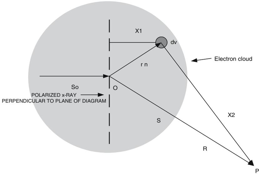
**Fig. A.1.**  $\mathbf{S}_0$  and  $\mathbf{S}$  are directions of incident (plane polarized) and diffracted X-ray from the volume element  $dv$  of the electron cloud.  $\mathbf{r}_n$  is the position vector of volume element  $dv$  having charge  $\rho dv$ .  $X_1$  is the distance of the volume element  $dv$  from the plane-polarized X-ray wave and  $X_2$  is the distance of the point of observation from the volume element  $dv$
