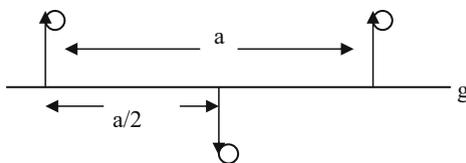
**Fig. 5.1.**  $a$  is the unit translational vector. The motif suffers a reflection on the mirror plane and undergoes a translation half the way.  $g$  the mirror perpendicular to the diagram and is known as the glide plane
