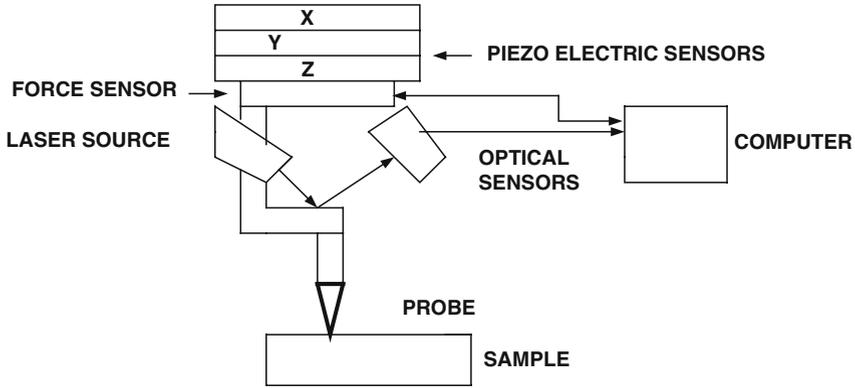
**Fig. 10.20.** The atomic force microscope. X,Y,Z are the piezoelectric sensors to control the motion of the probe over the sample in XYZ directions. Force sensor is to measure the force between the probe and the sample. (CPU) Computer – The computer is used for setting the scanning parameters such as scan size, scan speed, feedback control response, and visualizing images captured with the microscope
