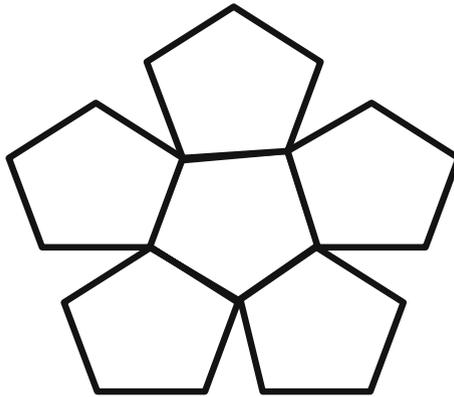
**Fig. 3.3.** It shows the impossibility of fitting regular pentagons having fivefold of rotation symmetry in condensed matter structure. Any such attempt will leave either voids or an overlap of the pentagons [2]
