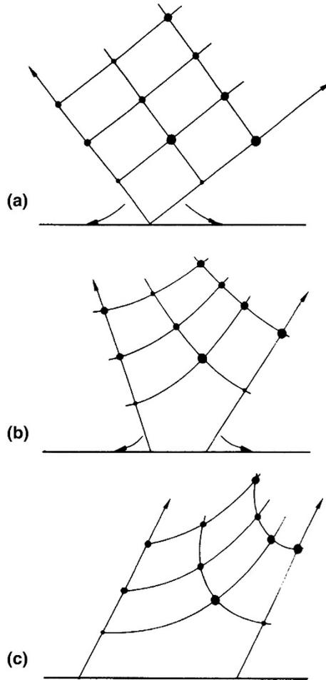
**Fig. 7.10.** (a) The weighted reciprocal lattice drawn say on a stretchable surface. (b) The axes are drawn from the origin away from each other with an intention to make them parallel to each other. (c) The axes are made parallel. The diffraction spots then resemble the Weissenberg photograph (replica) of Fig. 7.9, showing streamers and festoons (By courtesy of L.S. Dent Glasser)
