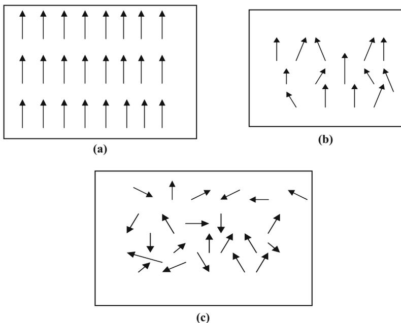
**Fig. 10.8.** (a) A perfect crystalline state of matter. Molecules preserve both positional and orientation order. (b) An intermediate state of matter. Molecules preserve orientation order but no positional order, and the matters preserve fluidity. A state of “anisotropic liquid.” (c) A totally disordered state of matter, for example, an isotropic liquid. The molecules preserve neither orientation nor positional order
