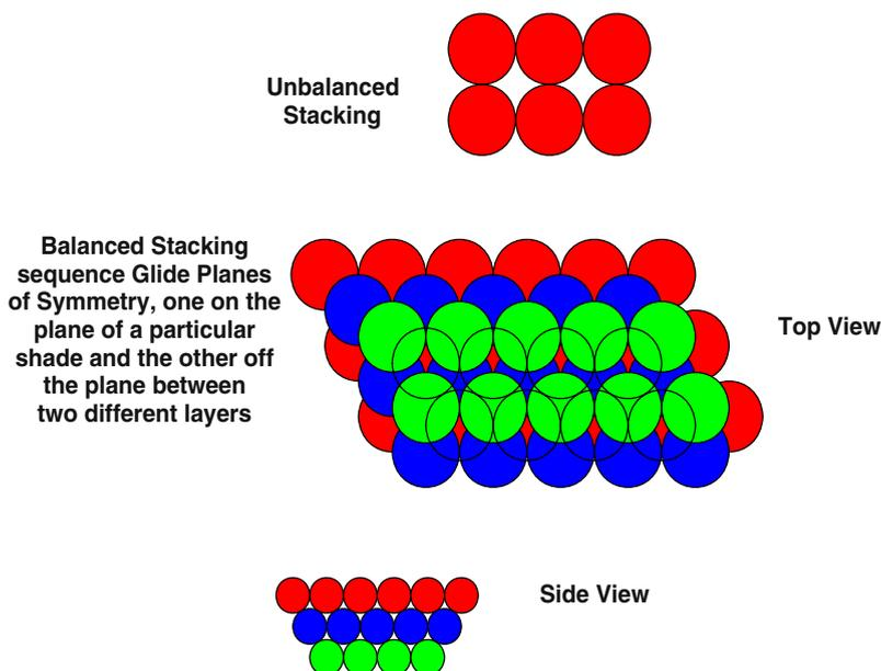
**Fig. 5.4.** The balanced stacking sequence of Billiard balls: *red* is the first layer, *blue* the second, and *green* the third. The fourth layer shown by open circle is the repetition of the first layer, that is, it can stay exactly over first layer. Each layer of first to third has suffered a glide in the plane over them
