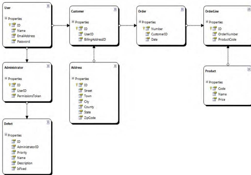
Figure 8-7. The LINQ-to-SQL mapping of the e-commerce tables, generated in seconds
