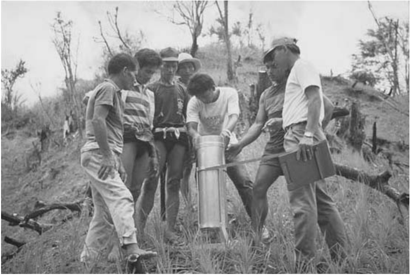
Plate 17 Installing rain gauge in kaingin .
