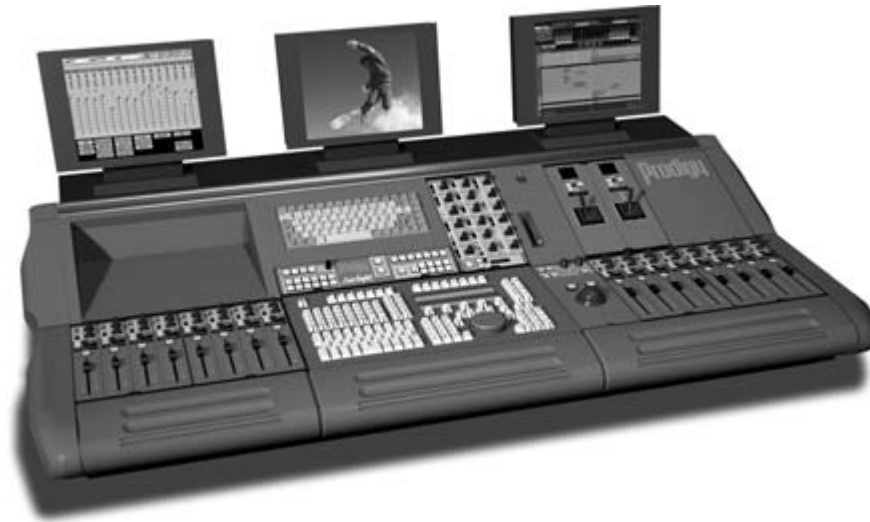
Figure 5.16 Audio control boards vary from small portable boards ( top ) for field and postproduction facilities to large multi-input and multi-output boards ( bottom ) for motion picture mixing theatres and music recording studios. (Courtesy Fairlight USA, and Mackie Designs, Inc.)
