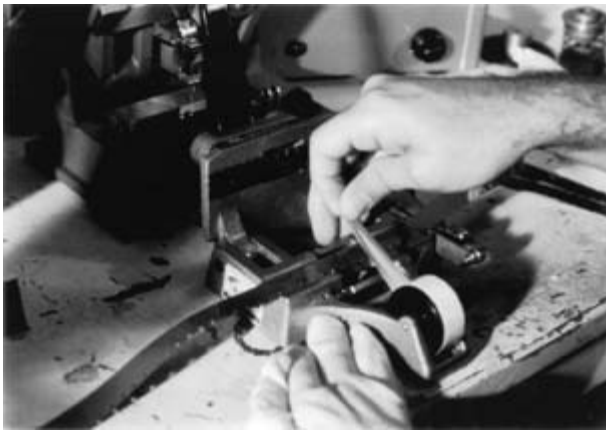
FIGURE 11.5 A splicer used to edit sound fullcoat film and workprint film uses a wide clear or opaque tape stretched across the film. The handle is brought down, sealing the tape and punching holes in the tape that is lined up with the sprocket holes in the film.
