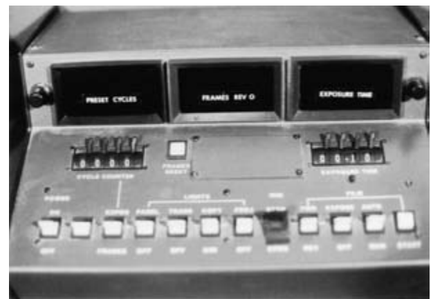
Figure 12.6 The control box for an animation stand provides the operator with the means of presetting the number of frames to be exposed on each cel, the exposure time, and all of the other camera controls such as iris setting.
