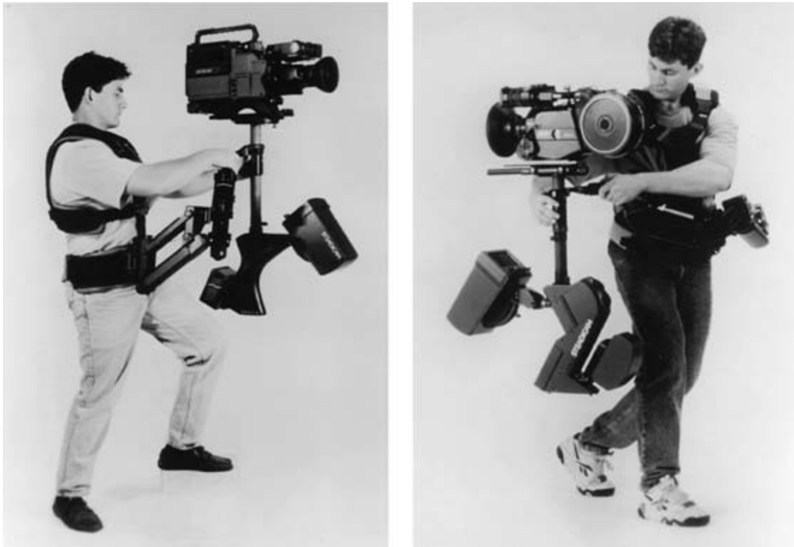
Figure 7.3A and B Body mounts are manufactured to carry either film or video cameras of all sizes. They are designed with a built-in spring and gyro system to maintain positioning on a level and even keel as the operator moves about the set. (Courtesy of Cinema Products.)
