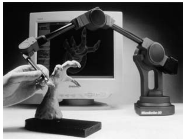
Figure 12.7 One of the methods of converting a solid object to a digital form is by tracing that form using a 3-D digitizer. The operator traces over all key surfaces of the object with a stylus until a full 3-D image has been transferred to a digital file. (Courtesy of Immersion Corporation.)
