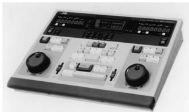
Figure 10.10 A linear editor controller controls tape decks of quality lower than the original or final format. In many cases a cuts-only editor, rather than an editor, allows dissolves or other effects. An off-line editor may become an on-line editor if the edit controller is used to control the highest-quality level desired by the producer. (Courtesy JVC.)
