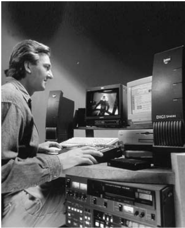
Figure 10.5 A nonlinear editing station consists of a series of monitors for viewing and hearing the material being edited and a computer to store and manipulate the footage. The footage is not actually cut and spliced, but is stored in the computer's memory in the order determined by the editor. Changes may be made quickly, easily, and many times over without damaging the original footage. Once the final edits are satisfactory, the final production can be fed out to either film or videotape for distribution. (Courtesy Scitex Digital Video.)
