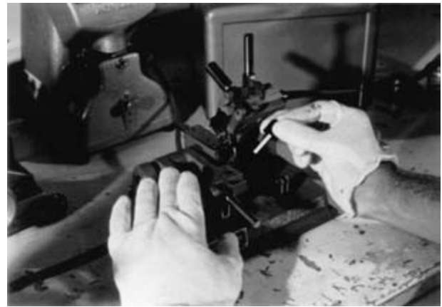
FIGURE 11.6 A splicer used to edit film to be projected or to assemble "A" and "B" rolls is called a hot splicer. A heating element built into the metal base of the splicer warms the deck of the splicer so that as soon as the acetone is applied to the joint between the film segments, the splice will quickly and permanently bond to create a secure splice. Separate magnetic film tracks are sometimes slugged or interspersed with clear leader, which is completely transparent film with no oxide coating. Using clear leader between recorded sounds is less expensive than using magnetic film, and it also clearly identifies where recorded audio occurs on the roll. Slugging with clear leader simultaneously on all edited sound tracks prevents any continuation of ambient noise or "room tone" and results in patches of completely silent or dead audio. Thus clear leader should only be used with tracks that will eventually be mixed with others.
