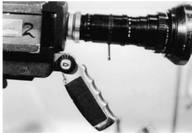
Figure 7.2 The smallest and most flexible camera mount is a pistol grip mounted on either the camera body or the lens. Using such a mount requires upper-body strength, since all of the weight of the camera and lens rests on the operator's shoulder and right hand. Much practice is necessary to learn to hand hold a camera in order to provide a steady, unwavering shot.
