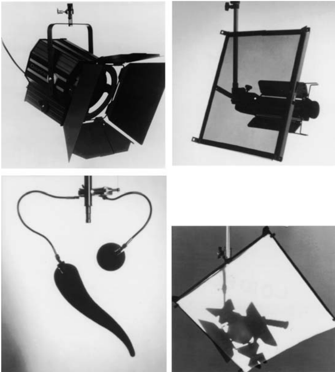
Figure 6.9 The control and shape of light as it falls on the set may be controlled by barndoors mounted on the front of the instrument, by reflecting light from a light surface such as an umbrella, or by placing scrims, flags, and diffusers between the lamp and the subjects. (Courtesy of Colortran and Lowell Light.)
