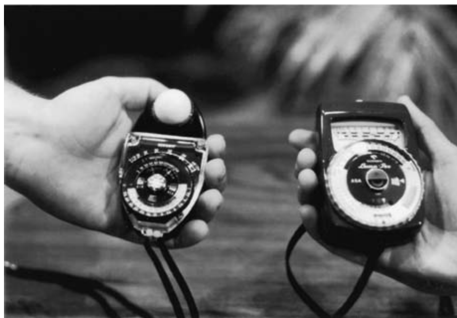
Figure 6.14 Handheld light meters may be designed for different functions. The one on the left is designed primarily to read incident light, and the one on the right is designed to read reflected light, although both meters will read either incident or reflected light.
