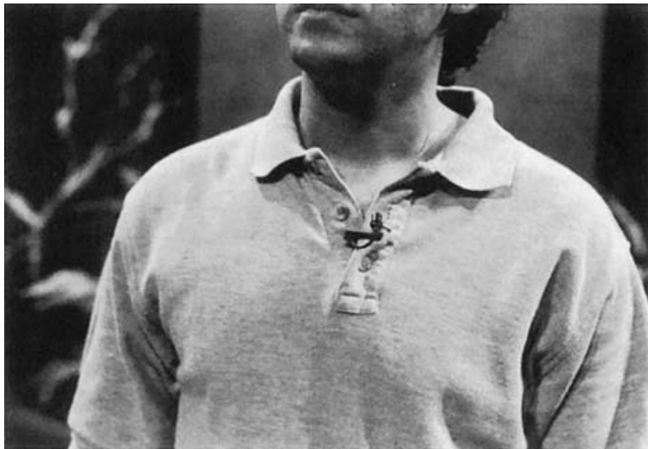
Figure 5.6 A lavalier microphone is designed to be clipped to the clothing of the person speaking. The design of a lavalier compensates for the microphone resting against the chest of the speaker, and the microphone is located below the speaker's mouth. A lavalier should not be used as a handheld microphone away from the body.
