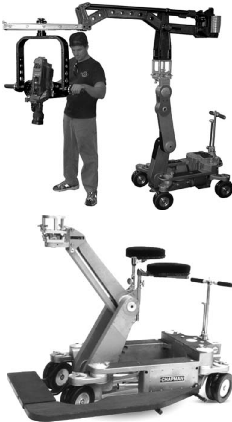
Figure 7.5A and B Dollies are constructed in a variety of shapes and sizes. These two are designed to be operated by hand, rather than motorized. The dolly in the top photo is designed with the camera mounted in a yoke and with the operator and grip moving the camera and dolly as needed. The dolly in the bottom photo is designed for the camera operator to ride seated. (Courtesy of Chapman/Leonard Studio Equipment.)
