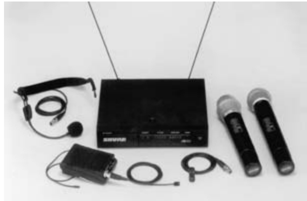
Figure 5.7 A wireless microphone may be designed as either handheld, a lavalier, or on a head-mount. The transmitter may be built into the base of the handheld microphone, or the lavalier and head-mount may be connected to a small transmitter fastened to the body of the performer. (Courtesy of Shure.)
