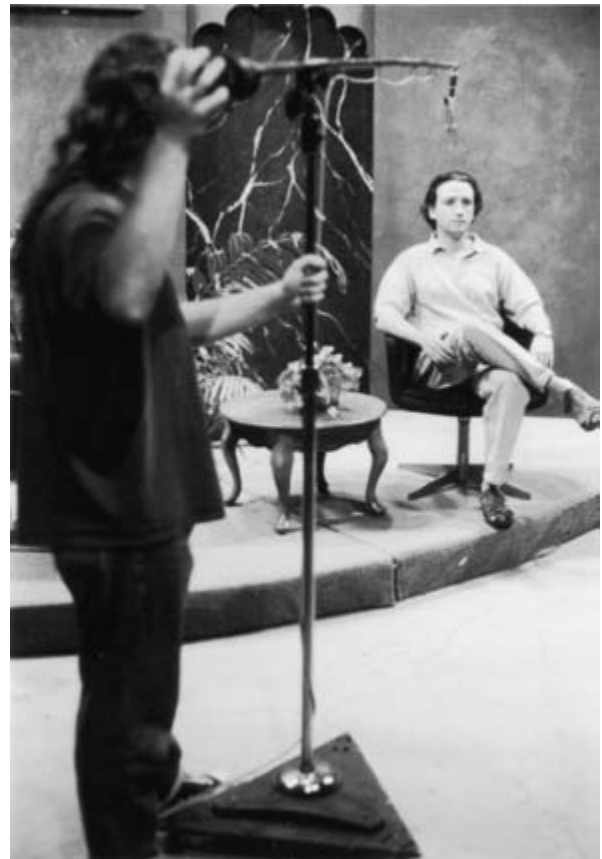
Figure 5.8 A giraffe microphone is a small boom generally used to pick up the voice of one or two persons in fixed locations.
