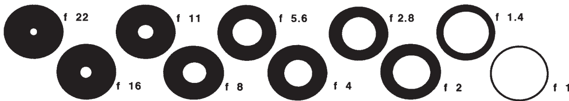
Figure 7.10 The numbers designating f-stops seem to act in reverse to their actual function. A small number, such as f 1.4, actually is a relatively large opening in the aperture, but f 22 is a relatively small opening, allowing very little light to enter the camera.
