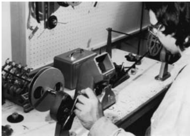
Figure 10.17 The basic film-editing bench consists of a pair of rewinds, a viewer, a synchronizer, and a supply of reels and spacers for the rewind shafts.
