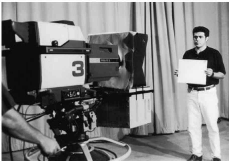
Figure 6.2 With the proper filter placed between the video camera lens and pickup chips or tubes, the camera's internal circuits will automatically white balance when focused on a pure white card and when the white balance switch is thrown. Film camera white balance is dependent upon the type of film stock and filter arrangement, not the camera or the camera's internal operation.
