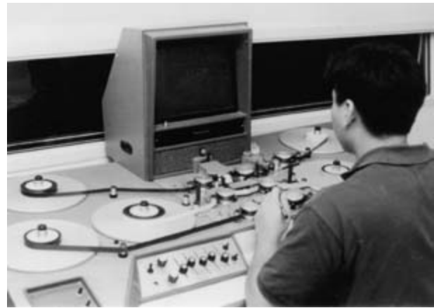
Figure 10.13 A flatbed film editor allows the operator to work with two sound tracks and the picture track simultaneously while viewing the picture on the screen. The tracks can be adjusted to sync with the picture while editing.
