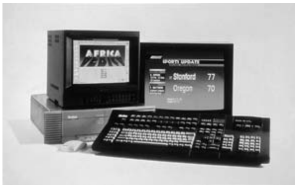
Figure 9.7 A character generator (CG) is a relatively simple computer graphics machine designed to create lines of type, including numbers, and simple color graphics backgrounds or lines of type to be keyed over other video frames. (Courtesy of Scitex Digital Video.)
