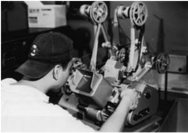
Figure 10.19 The upright Moviola editor has been the standard professional editing tool for many years. It has become less popular as the use of flatbed editors and posting film on video has increased.
