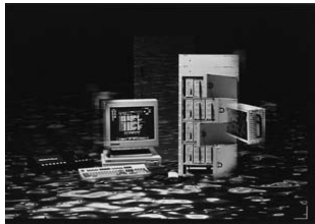
Figure 8.11 A video server that is designed to record and play back digital video/audio cuts on a nonlinear basis. It emulates videotape recorders, cart machines, and video storage systems. (Courtesy of Philips Broadcast Television Systems Company.)
