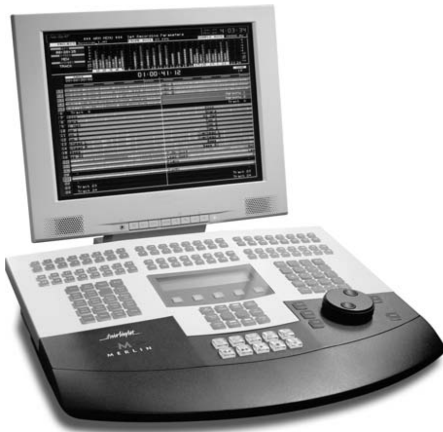
Figure 5.19 A digital audio workstation (DAW) is designed for quick editing for talk radio, call-in clips, news actualities, promotional announcements, and commercials. It is designed to edit like a word processor with cut/copy/paste and precision scrubbing functions. (Courtesy Fairlight, USA.)
