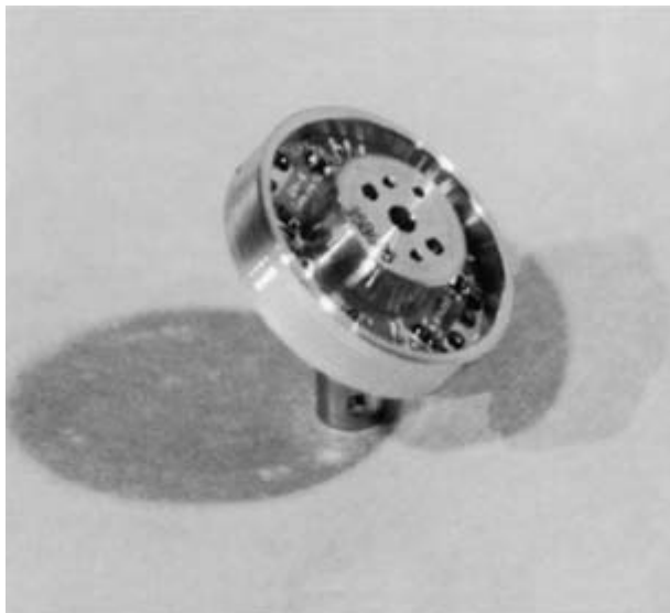
Figure 8.8 The video head of a helical recorder contains from two to eight different recording or erasing heads depending on the complexity of the format.
