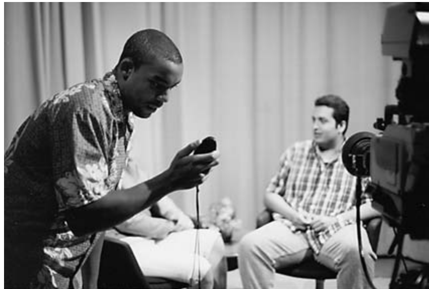
Figure 6.16 To take a reflected light reading, the meter is held close to the camera and pointed at the major subject. A narrow-angle meter provides the most accurate reflected meter reading.
