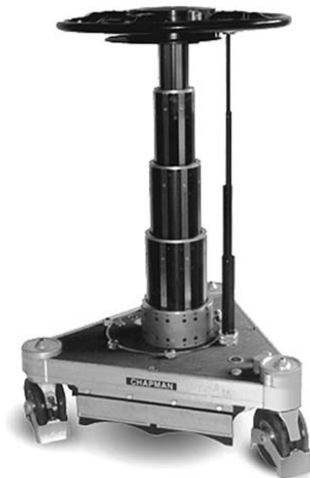
Figure 4.9 A studio pedestal is designed to allow the heavy weight of a studio camera, lens, and prompter to be moved about the studio with relative ease. The direction of the wheels under the skirt of the pedestal can be changed to allow the camera to be guided in any direction. The vertical pedestal column is counter-weighted or controlled by compressed air to allow the operator to raise or lower the camera easily and smoothly. The pan head is mounted on the top of the pedestal column. (Courtesy Chapman/Leonard Studio Equipment, Inc.)
