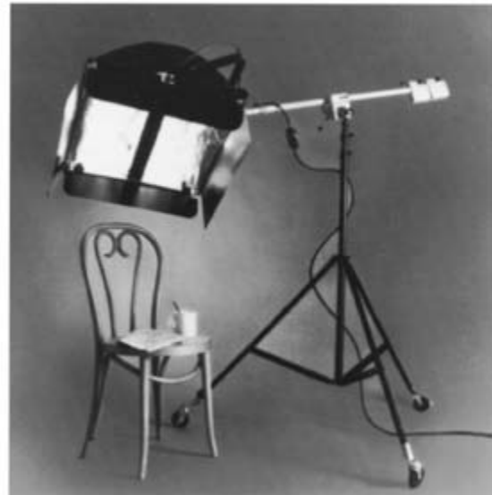
Figure 6.8A and B The design of portable light fixtures allows them to be mounted on floor stands, anchored by sand bags, hung from doorways, or clipped to other handy positions on the set. (Courtesy of Lowell Light and Colortran.)
