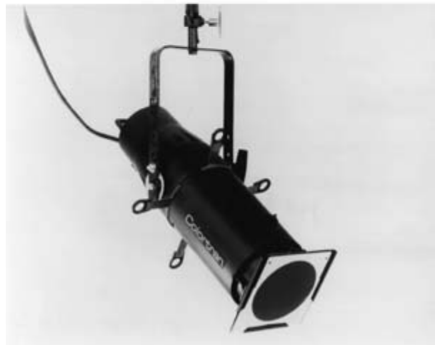
Figure 6.4A and B The light pattern from a Fresnel lighting instrument is controlled by moving the lamp inside the fixture closer or farther away from the stepped lens in the front of the instrument and by adjusting the barndoors mounted on the outside front of the lamp (top). The light pattern from an ellipsoidal lamp is controlled by adjusting shutters mounted inside the case of the lamp between the lamp and the front lens. Barndoors also may be mounted on ellipsoidal lamps (bottom). (Courtesy of Colortran.)
