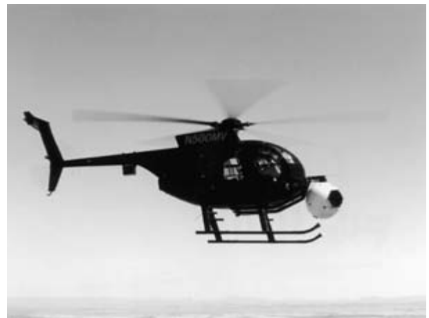
Figure 4.8 Among many other means of mounting either film or video cameras is the gyroscope mount, which can be mounted on an airplane, helicopter, or any moving vehicle. The stabilizing system provides a solid, smooth picture, and the operator inside the vehicle can pan, tilt, and zoom the camera as the shot requires.
