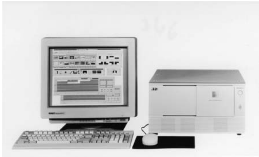
Figure 10.7 The screen of a nonlinear editor reveals the types of transitions available, the segments available to edit, the sound in visual form, time-code information, and running times of the production. Depending on the brand and model of editor, other characteristics of controls also may be visible on the screen. (Courtesy of Apple Computer.)
