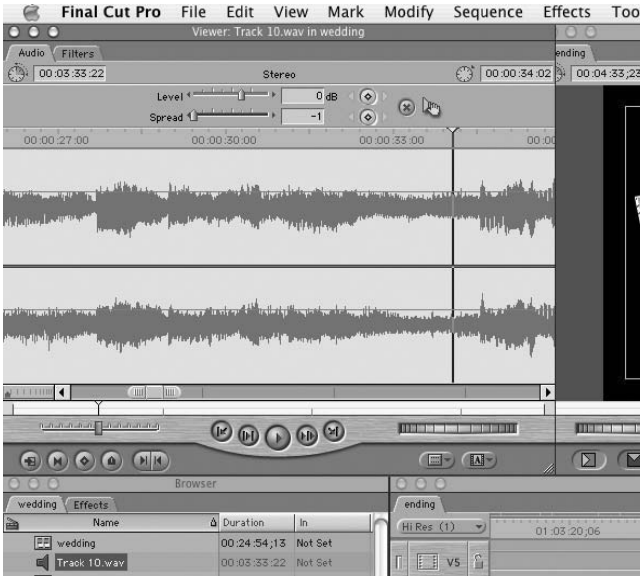
FIGURE 11.1 The screen on a computer running a digital audio editing program shows what the sounds look like in various formats. When editing, an audio editor visually cuts, pastes, and modifies the virtual files as if they were a part of word processing.
