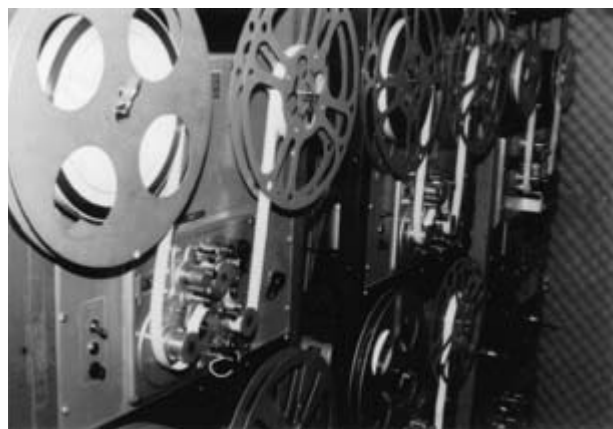
Figure 10.14 Fullcoat players and recorders are designed to keep a series of reels of sound tracks synchronized with the final edited workprint during the mixing and dubbing process.
