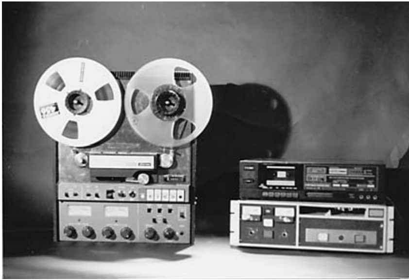
Figure 8.3 The common analog audiotape decks are: \frac{1}{4} -inch reel-to-reel, broadcast cartridge, and a standard \frac{1}{2} -inch cassette deck.
