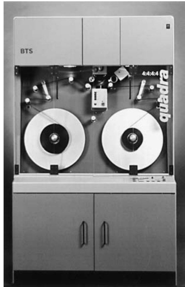
Figure 10.20 A CCD telecine film-to-video converter. Each film frame is scanned individually, allowing for color correction and filtering in real time as the film is converted to a digital signal. (Courtesy of Philips Broadcast Television Systems Company.)
