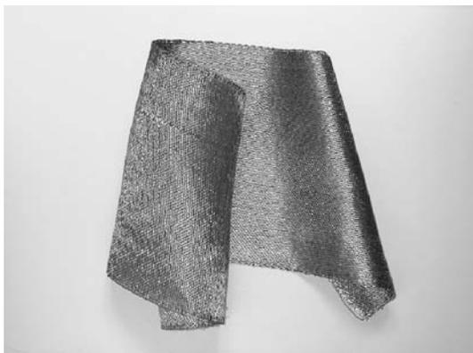
**Fig. 19** 8HS fabric made of a very thin SA fiber (diameter: 7~8  $\mu\text{m}$ )
