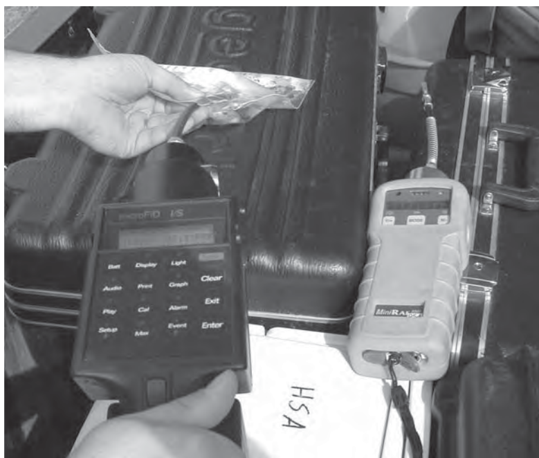
Figure 6.1 Flame ionization (left) and photo ionization (right) detector screening for VOCs.
