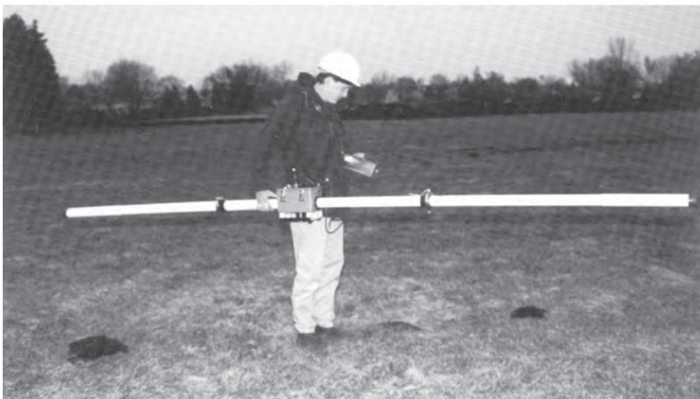
Figure 6.2 Magnetometer survey (provided by PEER Environmental, Inc.).
