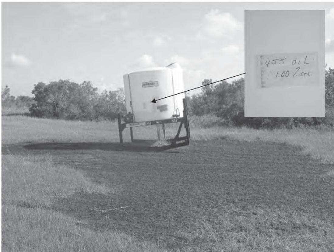
Figure 6.8 Damaged tank containing 455 oil (insert) and soil staining and stressed vegetation due to the release (provided by Derrek Verlaan).
